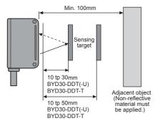
2. Install a target at sensing position and adjust the sensor to right and left or up and down to be at the right angle against the optical axis and fix it at stable operating position.
