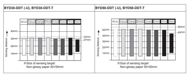
1)This model is photoelectric sensor with stable convergent detection type, therefore it is not affected by color or material within the range of sensing distance as specified in chart.
