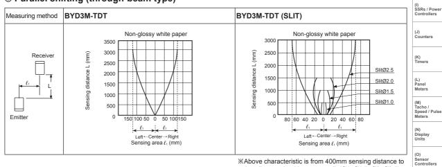
XAbove characteristic is from 400mm sensing distance to install transmitted beam type slit (Ø1, Ø1.5, Ø2, Ø2.5).
