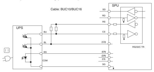
Connecting the BU70XS or BU606F by Cable or Connecting to Another UPS
