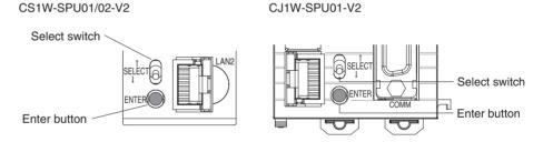
Setting Commands on the Select Switch The command number will be incremented when the switch is press up and decremented when the switch is pressed down.
