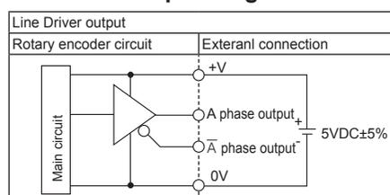
※All output circuits are same A,  $\bar{A}$ , B,  $\bar{B}$ , Z,  $\bar{Z}$  phase.
