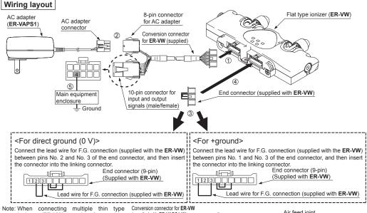
Note: When connecting multiple thin type ionizers (ER-VW) together for use, be sure to connect the supplied end connector to the linking connector (9-pin) for the final ER-VW in the series. In this case, be sure to connect the end connector according to the wiring process described above.
