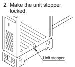
• Two installation positions are available for the unit mounting base so that the unit direction can be changed. Install the base at one of them.
