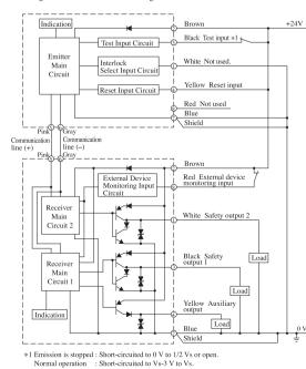
■Wiring to disable external device monitoring function Short-circuit the external device monitoring input to the
