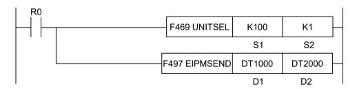
(Note 1) The figure above shows the case of specifying S1=K100 (Ethernet communication) and S2=K1 (connection No. 1) using F469 UNITSEL instruction.
