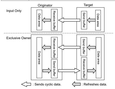
(Note 1) The transfer operations Data area>Send buffer and Receive buffer>Data area in each device are called "Refresh".
