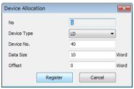
In this example, "Device Type = LD", "Device No. = 40" and "Data Size = 10".
