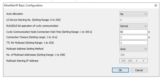
Change "Auto Allocation", "RUN / IDLE bit operation of cyclic communication", "Connection Timeout" as necessary.
