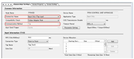
Once "Connection Name" is selected, "Communication Method" (Tag/Instance) will change. In this example, "Connection Name = Input Only (Tag type)".
