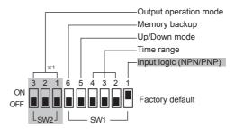
%1: Indicator model (FS5E-I4) does not have no. 1, 2, 3 of SW2 for output operation mode setting.
