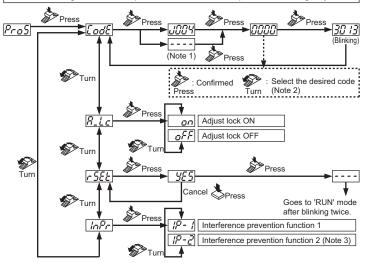
Notes: 1) When any code other than the codes given in the Code setting table below is used, ' - ' is displayed. The factory setting is 'ปบิบิน
