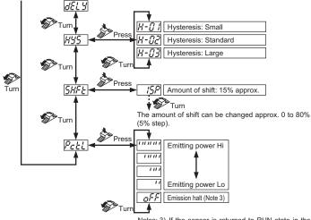
Notes: 3) If the sensor is returned to RUN state in the emitting halt condition, ' $\mathcal{E}_{-}o\mathcal{F}$ ' is displayed. The ' $\mathcal{E}_{-}o\mathcal{F}$ ' goes off when the emitting power is turned on.
