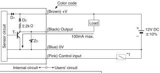
Symbols ... D<sub>1</sub>: Reverse supply polarity protection diode D<sub>2</sub> : Reverse current prevention diode Z<sub>D</sub>: Surge absorption zener diode Tr: NPN output transistor
