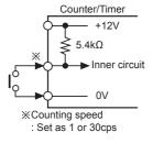
**%CP1**, CP2 (INHIBIT), RESET input part
