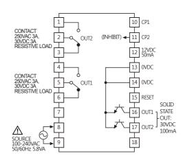
※INHIBIT: In case of timer mode, this terminal is for time hold. (voltage input (PNP): connect with 12VDC, no-voltage input (NPN): connect with 0VDC) (A) Photoelectric Sensors
