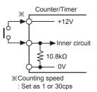
**%CP1**, CP2 (INHIBIT), RESET input part
