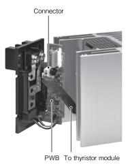
6. Thyristor module is seen, and detach thyristor module after removing D screw.
