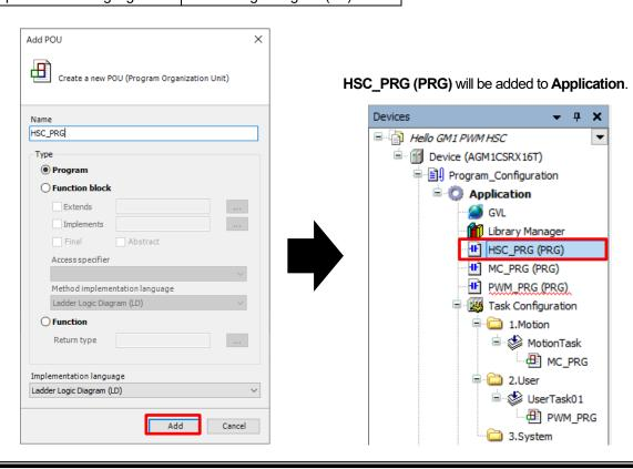
Drag and drop the HSC\_PRG (PRG) object added in Step 2 into 2.User in Task\_Configuration to add it to the task.
