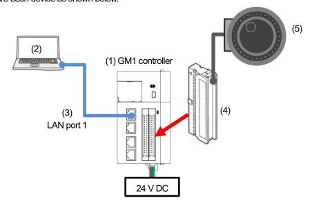
The GM1 controller uses high-speed counter input terminals to receive inputs from the high-speed counter. The line driver requires 5 VDC power supply. (Reference: The 5 V power supply of the FP0H CMO0 terminal can be used.)
