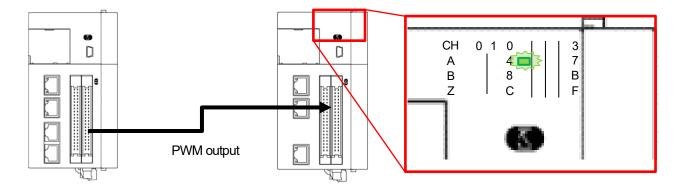
General-purpose I/O connectors Y4 to Y7 are assigned to the PWM output terminals on the GM1 controller. In this textbook, Y4 of Ch0 (one of the four channels) is used.
