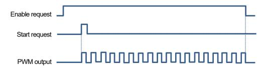
To update "Output frequency" and "Output duty ratio" during PWM output, write the respective values of "Output frequency" and "Output duty ratio" and then change the state of the start request bit from OFF to ON.
