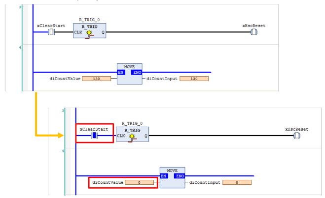
After checking is complete, set xClearStart to FALSE.
