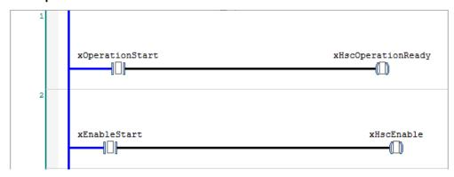
The operation request and enable request bits will be set to OFF and counter operation will be stopped. Then, even if the encoder is rotated, the count value will not be updated.
