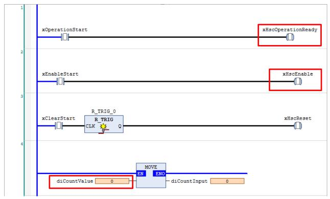
Even if the encoder is rotated in this situation, because the "Operation ready request" bit and "Count enable request" bit are set to OFF, any input from the encoder will not be accepted and the count values will not change.
