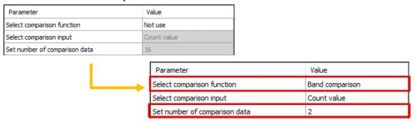
In **Comparison function**, setting items for the value entered in **Set number of comparison data** will be added. Here, two setting items "Comparison data 0" and "Comparison data 1" will be added.
