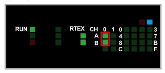
Because "2-phase input 4 multiple" is set, check that count operation is performed as below.
