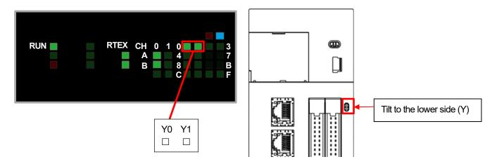
Rotate the encoder and check the status LED indicator when the count value is between 100 and 200. You can confirm that Y0 is lit.
