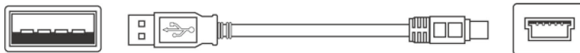
USB A type (male) - USB miniB type (5-pin, male) (PC side) (GM1 side)
