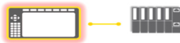
GP-S070-T9D6 CPU : Q02HCPU, Communication card : QJ71C24N
