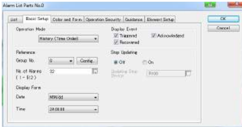
Setup of an alarm list part for displaying alarms in chronological order
