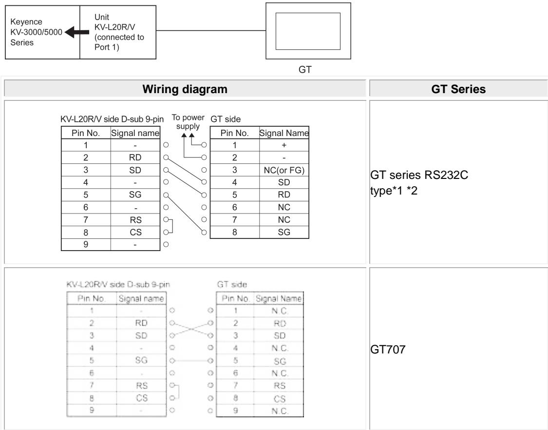
\*1: Although nos.6 and 7 of the models except GT01 are RS/CS, they can be used in the above connection.
