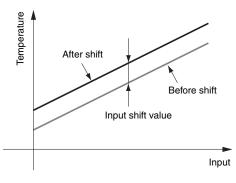
The value set for the temperature input shift is applied to the entire measurement range of the temperature sensor.
