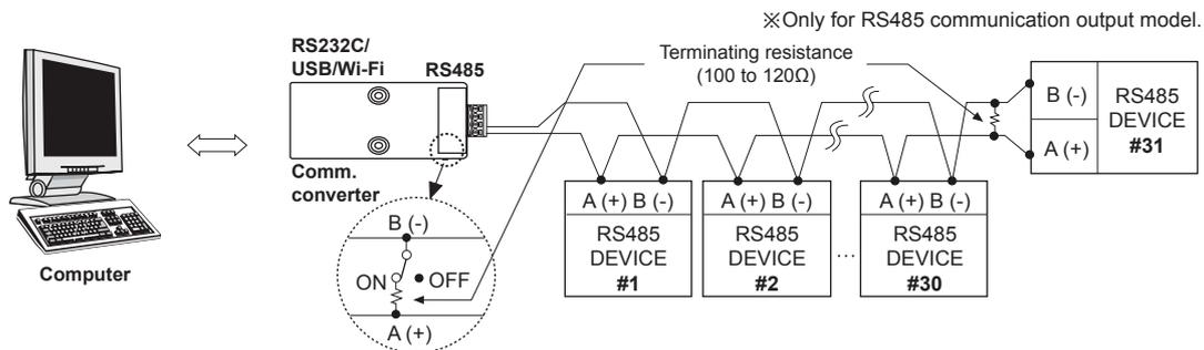
※ It is recommended to use Autonics communication converter;
