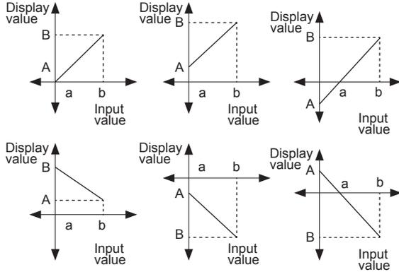
Display scale function is able to change display value for max./min. measured input by setting high limit scale [H-5C] and low limit scale [L-5C] in program mode.
