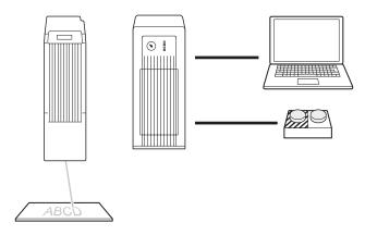
Controlling the laser marking system using a switch
