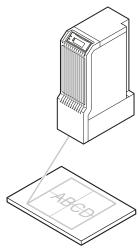
The guide laser indicates the marking image, the marking field, or masked objects, depending on your selection for "Guide laser display".
