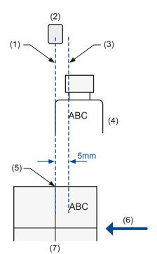
There is a distance of 5mm between the trigger detecting position and the marking data.
