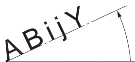
Straight line, left alignment
