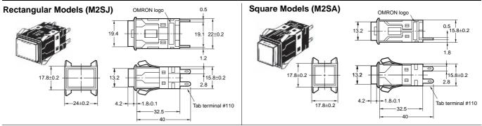
Note: Unless otherwise specified, a tolerance of ±0.4 mm applies to all dimensions. Recommended panel thickness: 1 to 4 mm
