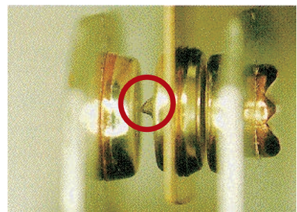
Contact transfer due to inrush current
