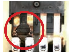
Short-circuiting between contacts of different polarity
