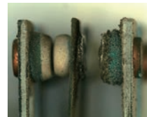
Corrosion due to nitric acid
