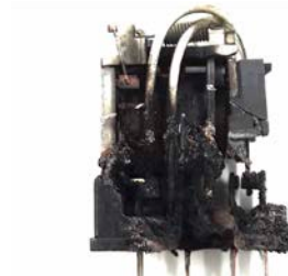
Burn damage due to insulation failure
