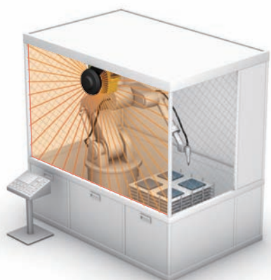
Fig. 1-5 Vertical Guarding Installation
