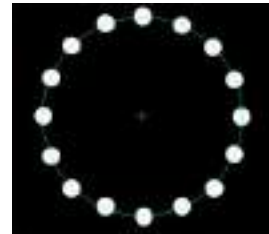
Measurement of approximate circle with multiple points
