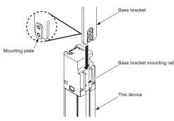
2. With the base bracket in firm contact with the device, tighten the two ultra lowhead hex socket bolts [M5 (length 5mm), opposing faces 3mm] that fasten the base bracket. Tighten to a torque of 3N·m or less.
