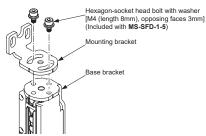
3. Install the beam adjustment mounting bracket on the mounting surface with a hexagon-socket head bolt (purchase separately)
