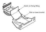
3. Install the intermediate supporting bracket on the mounting surface with two hexagon-socket head bolts [M5 (purchase separately)].
