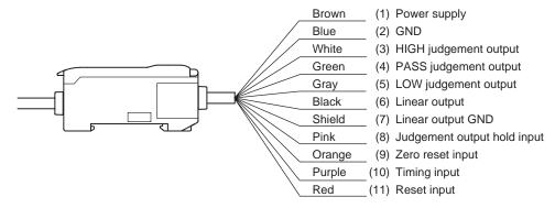
(1) A 12- to 24-VDC (±10%) power supply is connected to the power supply terminals. When using an Amplifier Unit with a PNP output, the power supply terminal is also the common I/O terminal for all I/O except for the linear output.
