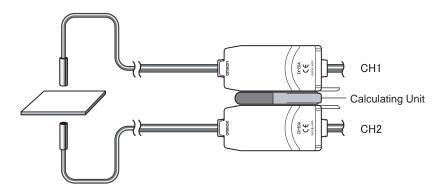
The calculation result is displayed on (i.e., output to) the CH2 Amplifier Unit. Connect the CH2 output cable to the external device to enable external control.
