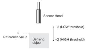
Using the Height of Sensing Object as the Measured Value with an Offset Set to 10
