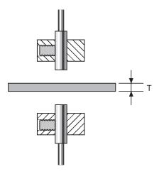
When the thickness is entered, the positional relationship between the Sensor Heads at that point will be registered. The thickness is measured based on the positional relationship of the Sensor Heads.
