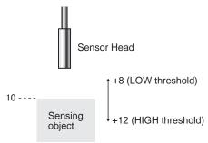
Example 3: Using Zero Reset to Measure Steps in Sensing Object (Zero Reset at Each Measurement)
