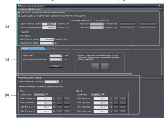
Set the operation command generator and conditions and also damping control conditions.
