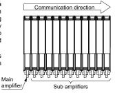
When this product and other products (e.g. fiber sensor amplifiers, pressure sensor controllers, etc.) are connected together in cascade, install those products so that they are in order of Group A, B, D and C as shown in the right figure. This product is included in Group D.
