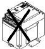
Horizontal installation of PLC main unit
