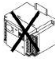
Installation getting the DIN rail upright
