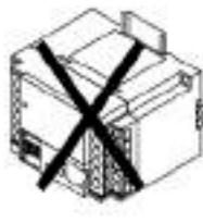
Installation getting the DIN rail upright
